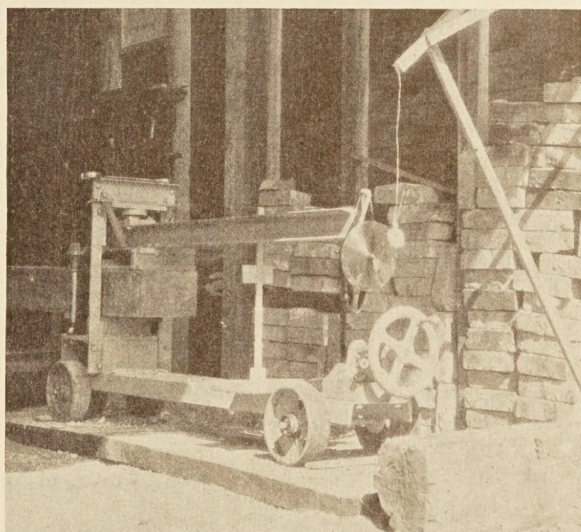
THE BEAM-TESTING MACHINE AND THE LOAD APPLICATION WERE CONTROLLED SO AS TO BE THE SAME ON ALL SPECIMENS, AND ALL TESTS WERE MADE BY THE SAME OPERATOR.
